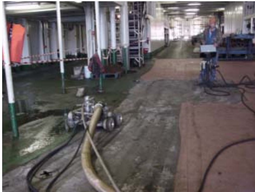
Figure 4. A second variation of the semi-automated tool is a crawler type device. This system has the added advantage of being able to do work on vertical surfaces.
