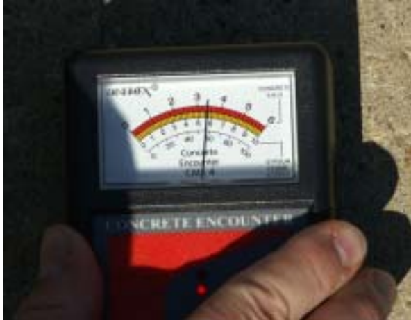
TEST ZONE #2 SpinJet with Vacuum Recovery – Pre-Test Moisture Reading Of 3.4% H 2 O.
