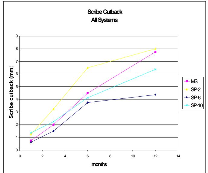
**GRAPH 3. COMPARISON OF SCRIBE CUTBACK RESULTS SORTED BY COATING SYSTEM FOR THE TEST BEAMS UNDER MARINE ATMOSPHERE EXPOSURE.**
