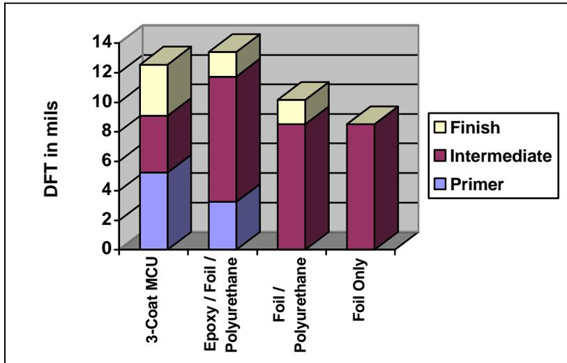
**GRAPH 1. FILM THICKNESS AVERAGES OF THE COATING SYSTEMS TESTED.**
