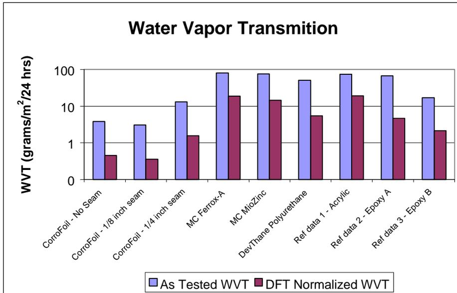
**GRAPH 9. COMPARISON OF WATER VAPOR TRANSMISSION RESULTS FOR VARIOUS COATING FILMS.**
